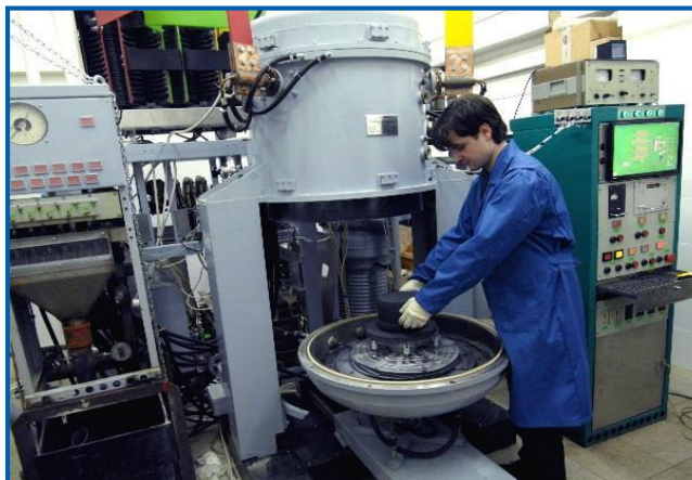
Vacuum furnace for high-temperature coating application
