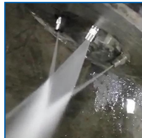
Plant for metall powder production by high-pressure spraying
